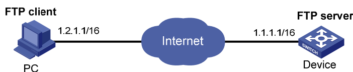
Figure 38 Upgrading using the FTP server
